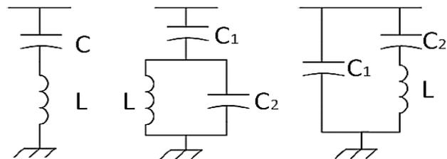
**Figure 1:** Different Filter Topologies (a) ST Filter (b) C Type Filter (c) CCL Filter [5]
