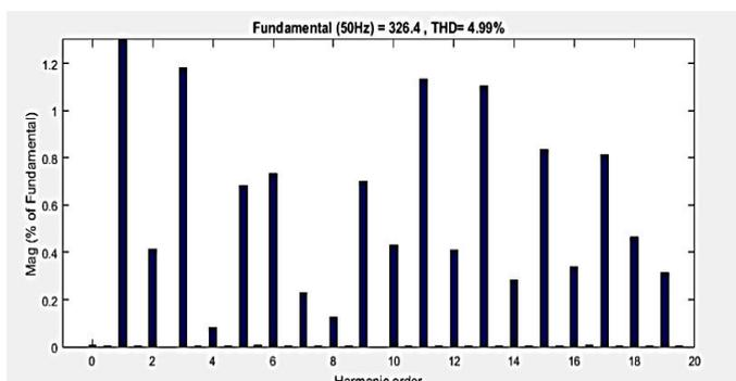
**Figure 8:** FFT Analysis of source current with Detuned filter
