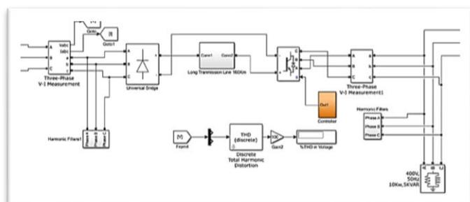
**Figure 7:** Simulink model of Detuned filter
